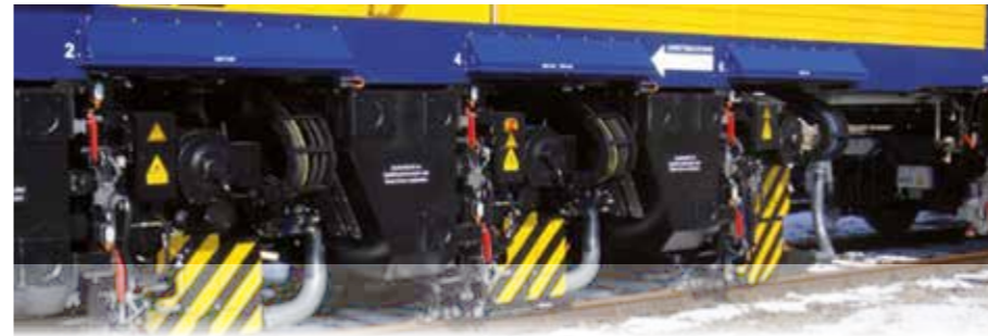
Camera-monitored rail track processing units.
