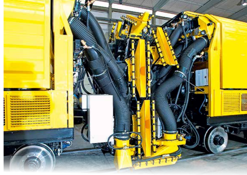
The "tunnel cleaners" regularly remove fine dust and coarse dirt from tunnels. Cameras monitor the cleaning units.
